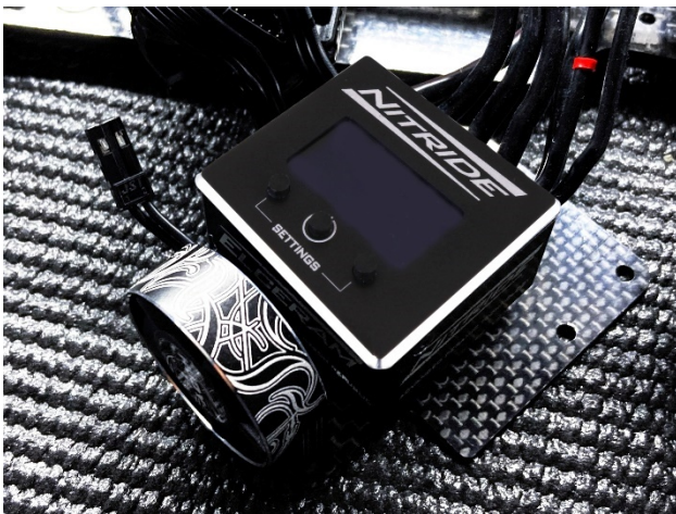
Example of NITRIDE installation into on-road car using the fan for use with the motor 4,5T on asphalt
