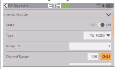
The Internal RF module supports 24 channels (CH1-8 / CH1-16 / CH1-24).
