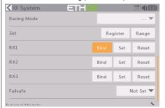
Move the cursor to RX1 [BIND], press it and repower the receiver.
