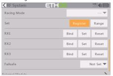
For TW Mode as an example, select the Set [Register] for getting the radio into Registration status in the RF System-Internal Module tool, then press the F/S button on the receiver and power the receiver on.
