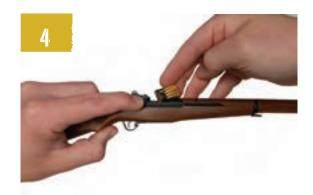
Pull back on bolt to reveal clip loading area. Insert clip with dummy rounds facing the barrel. Push down until the bolt is clear and able to slide.
