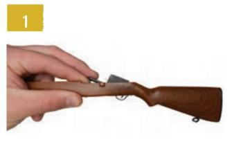
Place trigger housing group (A) in stock (B) Housing group has tabs on both ends to hold it in place.
