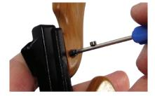
Place stock (E) onto lower receiver (C) and screw into place.
