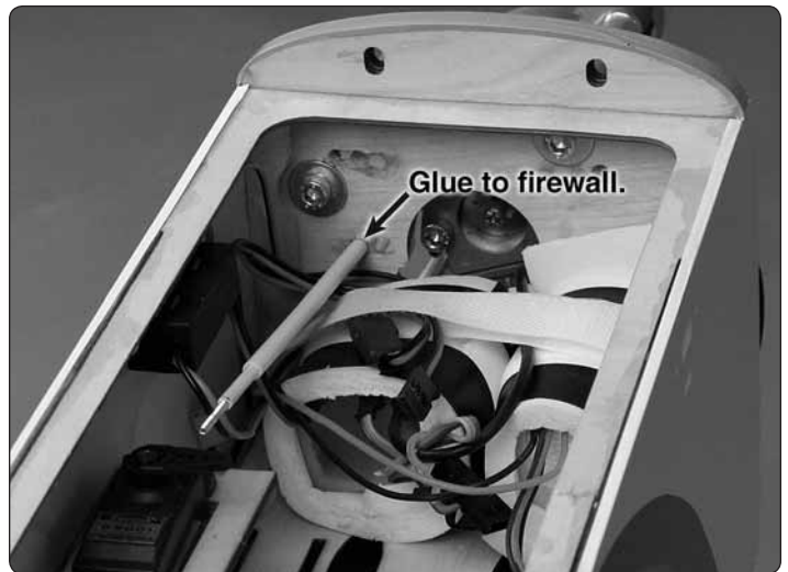
❑ 24. Install the outer pushrod.
