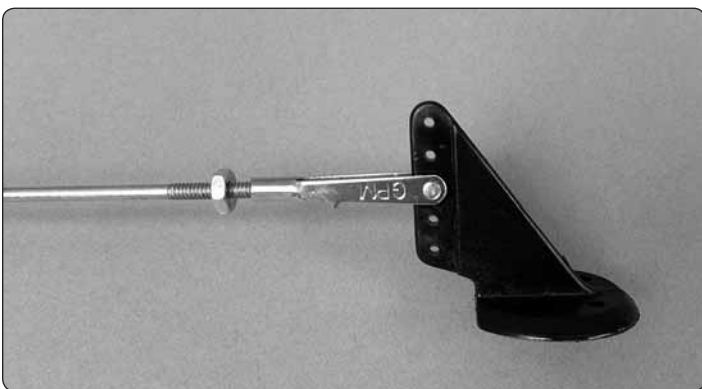
□ □ 9. Attach clevis to control horn.
