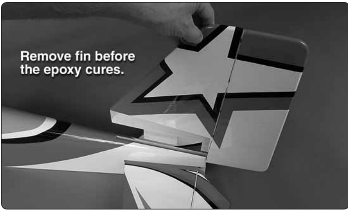
❑ 6. Use 30-minute epoxy to glue the stabilizer in the fuselage.
