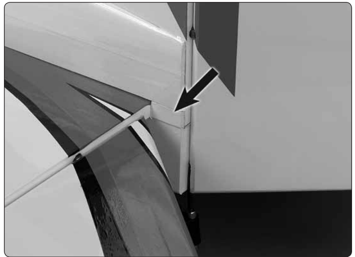
❑ 8. Glue the filler blocks on both sides of the fuselage.
