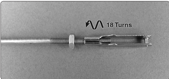
□ □ 8. Install the 4-40 threaded clevis.
