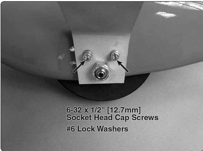
❑ 5. Install the wheel pants.
