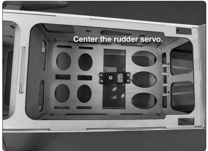
❑ 1. Install the rudder servo and plug it into the receiver. Temporarily plug the receiver battery into the receiver.
