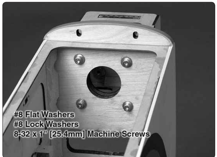
❑ 7. Attach the motor box to the firewall.
