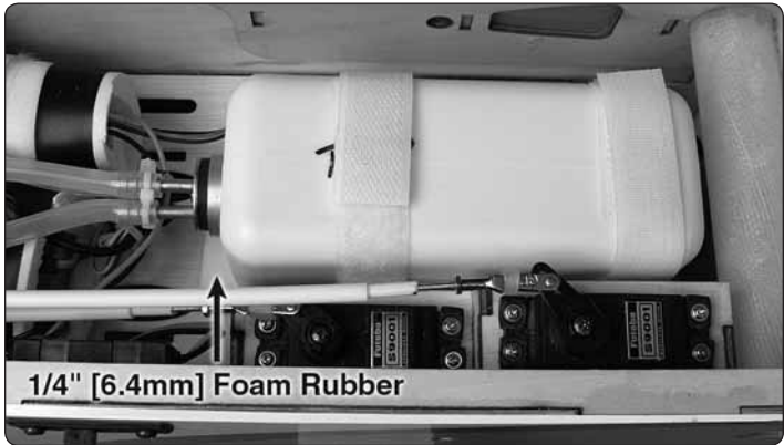
2. Secure the fuel tank in the fuselage.
