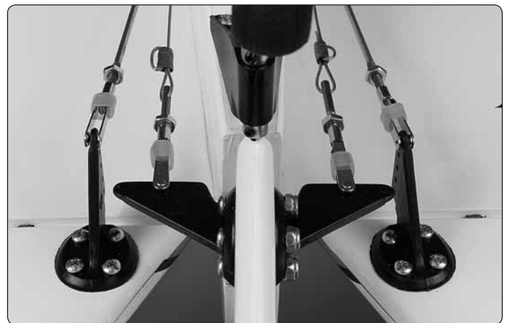
□ 13. Install the elevator control horns and attach the 4-40 clevises, nuts and retainers.
