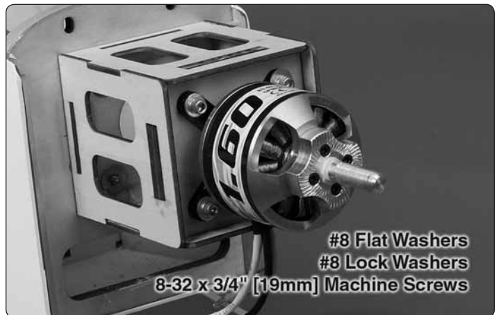
❑ 8. Install the RimFire 1.60 motor.
