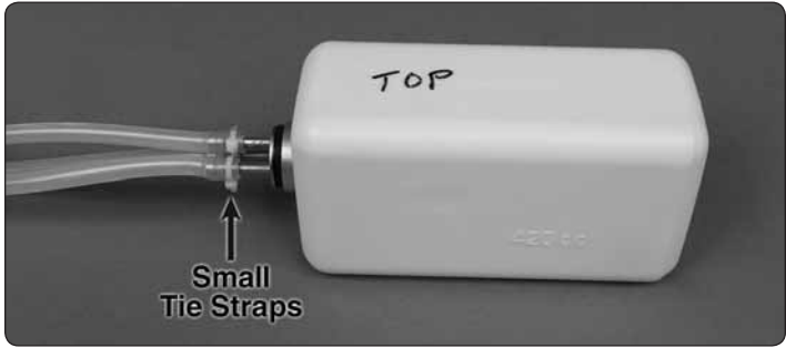
1. Install and mark the fuel lines: Vent, Carb and Fill.
