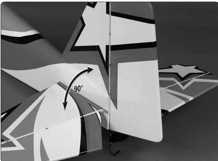
❑ 7. Use 30-minute epoxy to glue the vertical fin in the fuselage.
