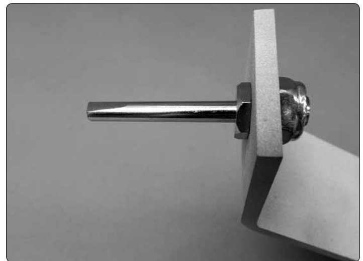
❑ 3. File a flat spot at the end of the axle.
