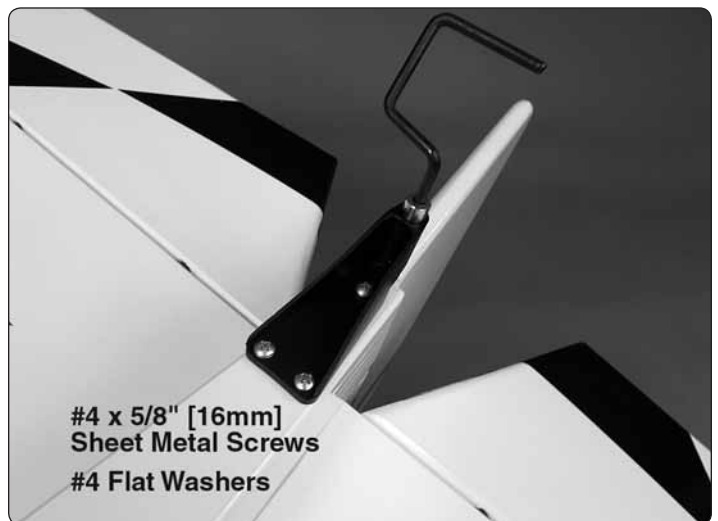
❑ 9. Attach the tail gear to the fuselage.
