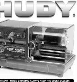
the tire truer to a 12VDC power source. If you are using a DC power supply, make sure it can supply at least 25A. If to use the slowest tool movement speed, connect the tire truer to a DC power supply that can supply at least 14-16V.
